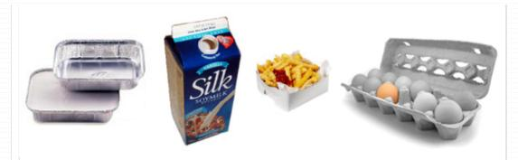
Laminating paper-based board with other materials creates boards with different qualities. These are known as composite materials e.g. – cereal packets, egg cartons, orange juice cartons, etc. A good example is foil lined board this has foil on one side of the board and is used for fast food containers to keep moisture an heat in.
